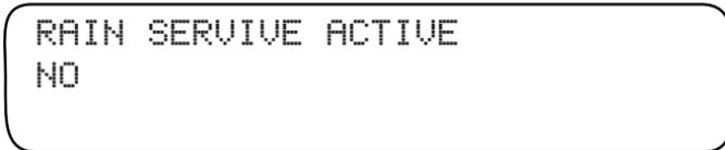
**NO** is selected by default. The display will automatically indicate **YES** when **Rain Service** has been activated.
